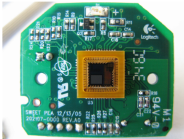
Figure 3 - Photo of PCB with CMOS chip from dismantled camera
