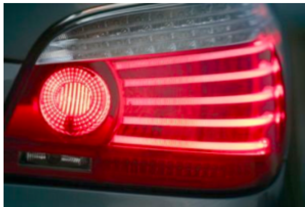
Fig. 8. Using the planar light guides in BMW 5
