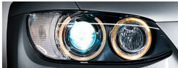
Fig. 7. The use of tubular light guides in the lamp Angel Eyes
