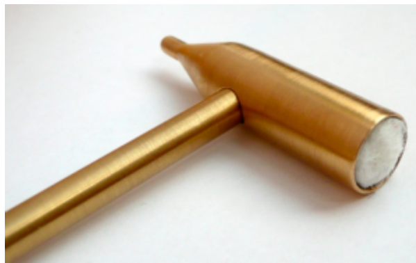
Fig. 5. Design of the double-sided test electrode.
