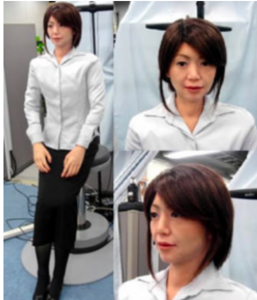
Fig. 3. Repliee Q2 is an upgraded version of Repliee Q1. The face of Repliee Q2 has become more humanlike. Furthermore, it has 13 DoFs in the head so that it can make some facial expressions and mouth shapes.
