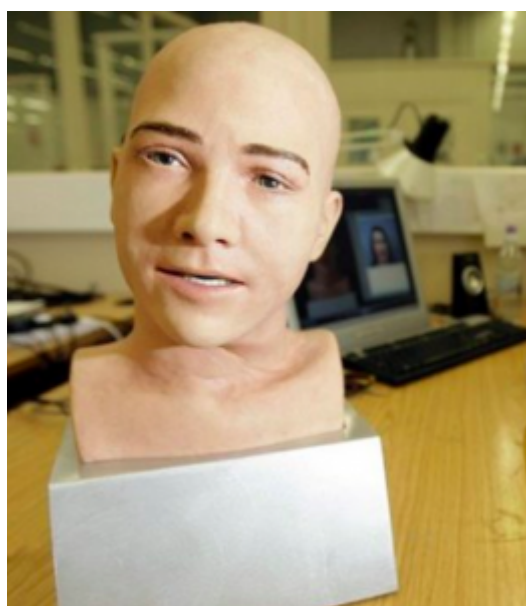
Fig. 1. Robot Jules is the first humanoid robot who can realistically mimic a real person's expressions, developed by HANSON ROBOTICS
