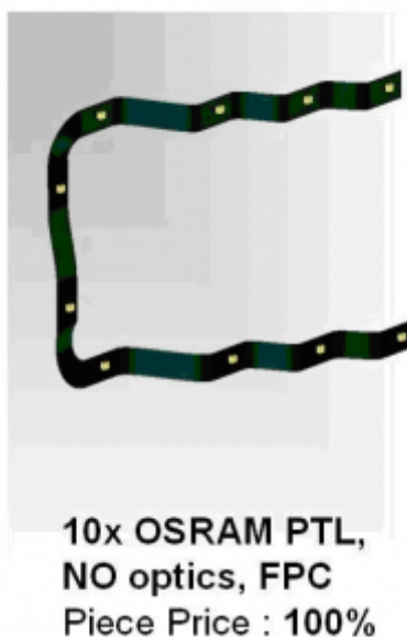
Fig. 8: Solution with LEDs placed on flexboard
