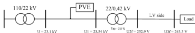
Fig. 4 Voltage in a low voltage network with the supply and distribution transformer 22/0,42 kV (transformer tap - 2,5%) with a connected PVE in the medium voltage network
