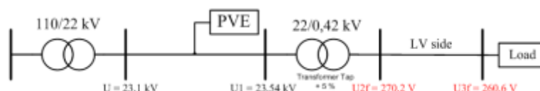
Fig. 3 Voltage in a low voltage network with the load and distribution transformer 22/0,42 kV (transformer tap + 5%) with a connected PVE in the medium voltage network
