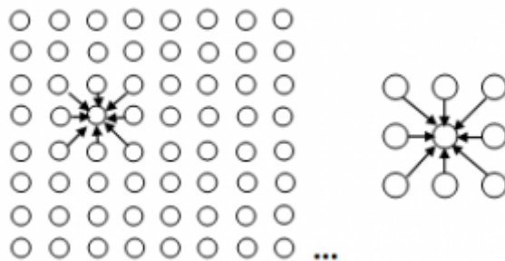
Fig.2 Considered fine-grained PGA architecture
