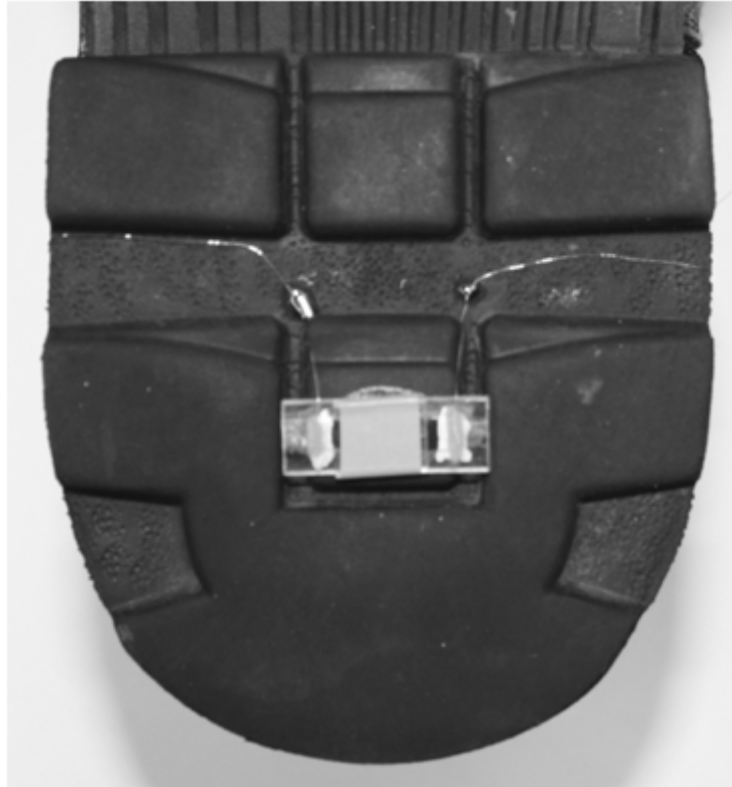
Fig. 2 MWCNT/TPU composite pressure sensor pasted to a shoe sole.
